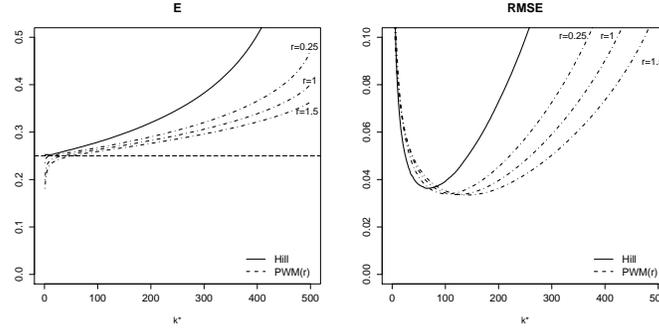
**Fig. 2** Simulated mean values (left) and root mean squared errors (right), as functions of  $k^*$ , of the estimators  $\hat{\gamma}_{k^*,n}^H$  and  $\hat{\gamma}_{k^*,n}^{PWM(r)}$ ,  $n = 500$ , from a Burr(0.25, -1) parent.
