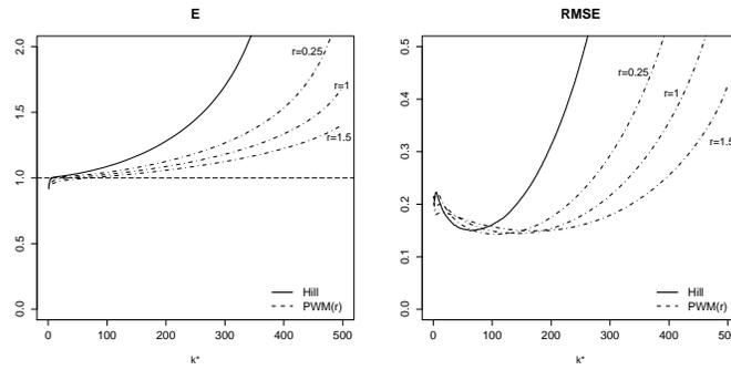
**Fig. 4** Simulated mean values (left) and root mean squared errors (right), as functions of  $k^*$ , of the normalized estimators  $\tilde{Q}_{k^*,n}^{W,H}(p)$  and  $\tilde{Q}_{k^*,n}^{PWM(r)}(p)$ ,  $n = 500$ , from a Burr(0.25, -1) parent.
